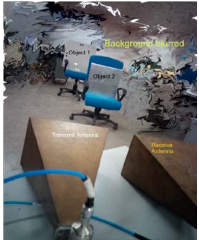
Figure 5 Transmit and receive antennas with test objects for detection
